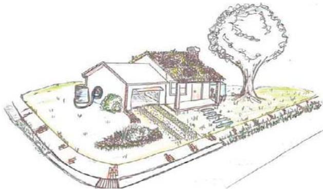
The advantages of using GSI in place of traditional storm water management controls are many and varied. When incorporated as part of the planning process, the result is wetland and riparian habitat protection, reduction of peak runoff flow and rate through the reduction of impervious surfaces, reduced risk of flooding,
