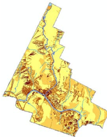
Figure 7: Map of Future Impervious Surfaces in Montpelier – Darker areas indicated greater volumes of runoff
