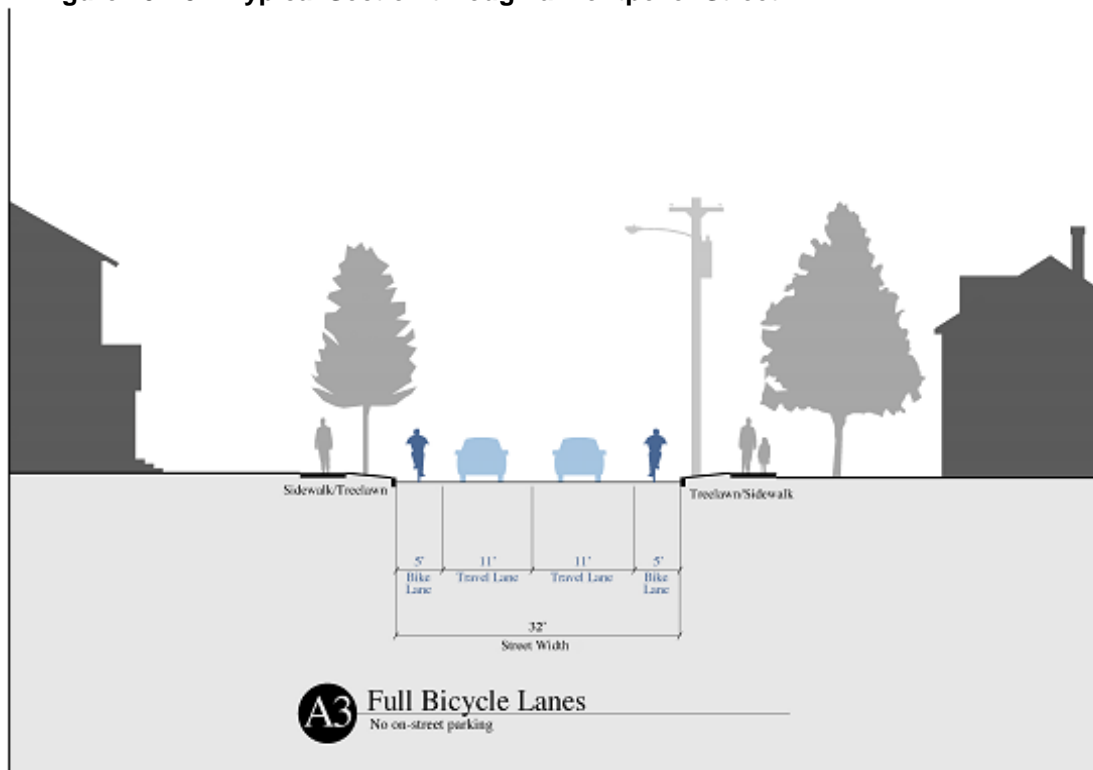
Figure 20 A3 – Typical Section through a Montpelier Street
