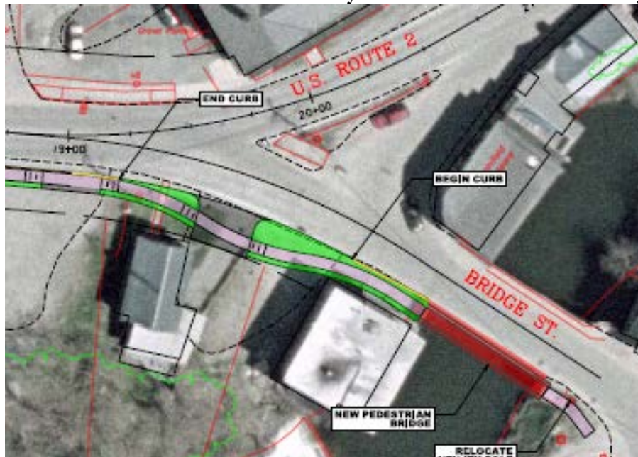
Illustration 4: Schematic Sidewalk Layout Close to Main Street Bridge
