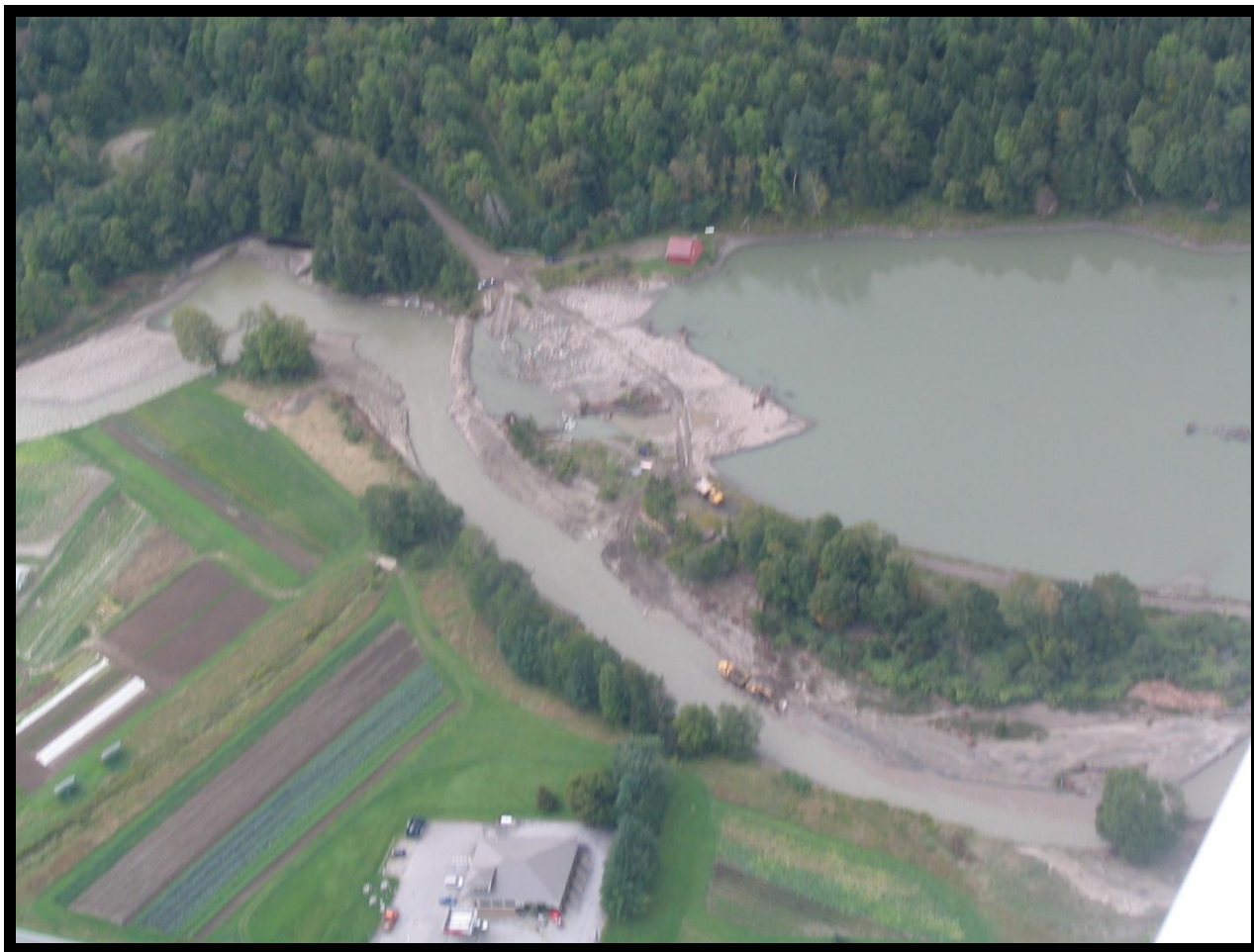
Figure 1 Sugarbush Snowmaking Pond. Damage after river avulsion after Tropical Storm Irene.
