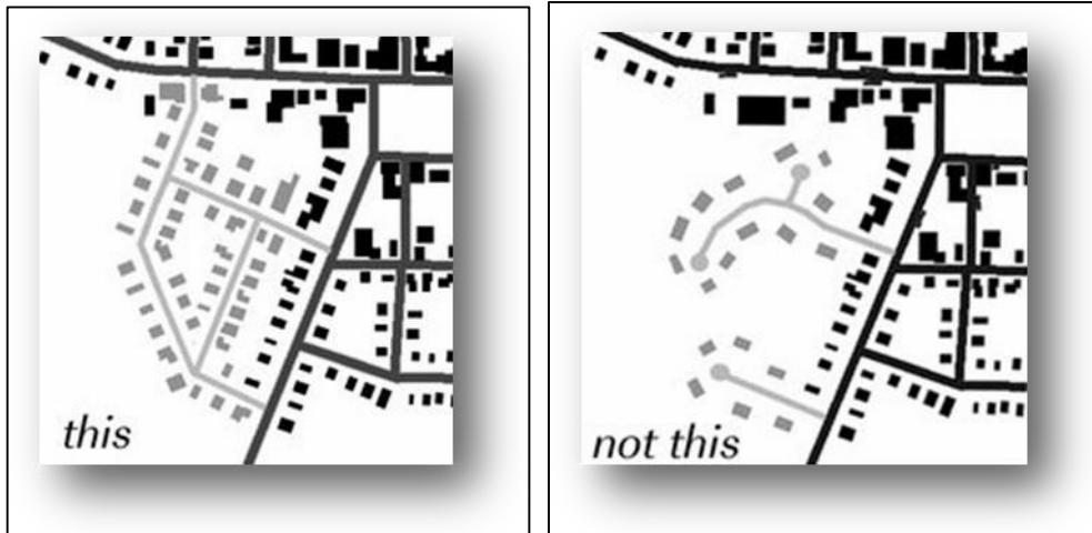
Figure 1: Connected Streets. The diagrams above illustrate two different traffic patterns created by new development (shown in light gray). The diagram on the left highlights several smart growth principles by integrating the new roads with the existing road and providing for a mixture of uses at a density consistent with compact development (Smart Growth Vermont).
