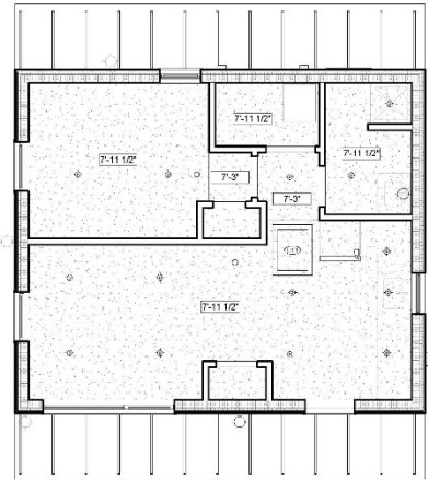
4 RCP - SECOND FLOOR Scale: 1/4" = 1'-0"
