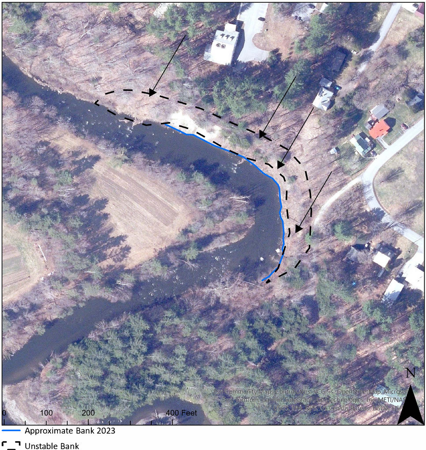
Figure 2: Aerial imagery with the approximate 2023 streambank outlined in blue. Black arrow shows areas that appear to have the most land movement. Dotted line highlights approximate area of current instability.
