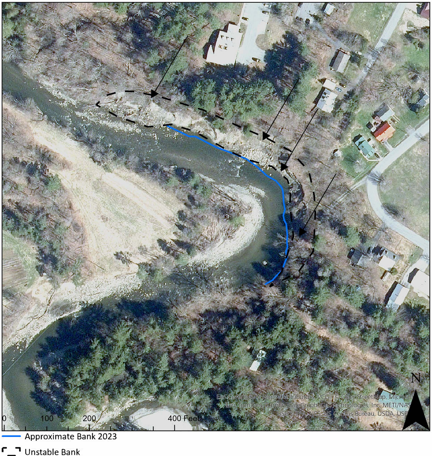
Figure 1: Aerial imagery with the approximate 2023 streambank outlined in blue to show movement. Black arrow shows areas that appear to have the most land movement. Dotted line highlights approximate area of instability.
