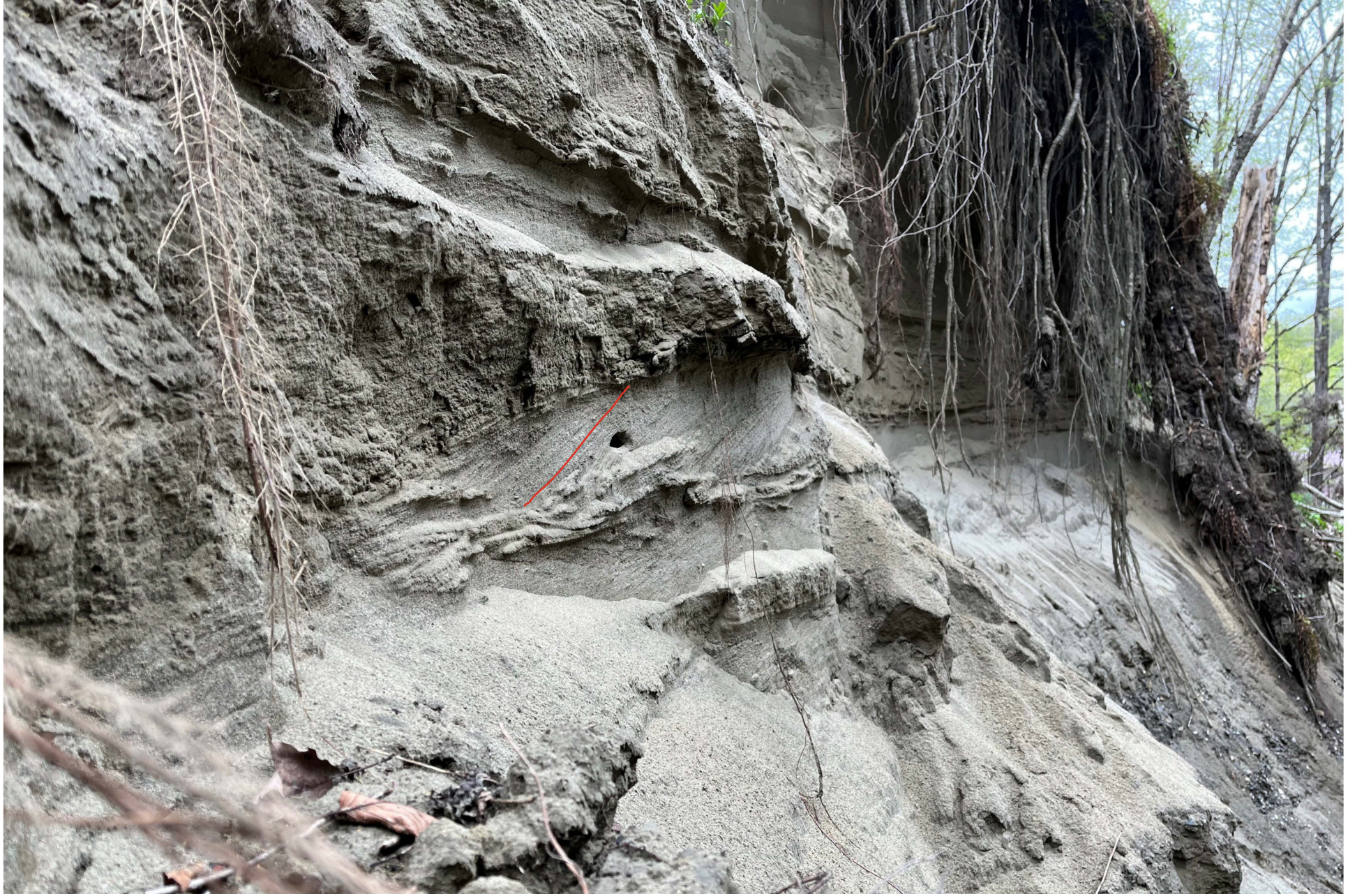
Figure 9: Photo taken on 5/8/2025 showing the variability in the depositional environments of the uppermost deposit. Despite the changing environmental conditions the deposit largely classifies as SP soils and coarsens upwards where some beds may classify as GM.
