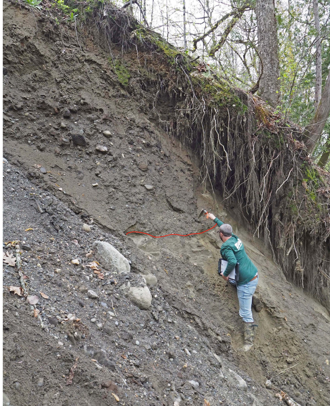
Figure 8: Photo taken on 5/8/2025 revealing wavy boundary between till and underlying glacial lake deposit (see line).
