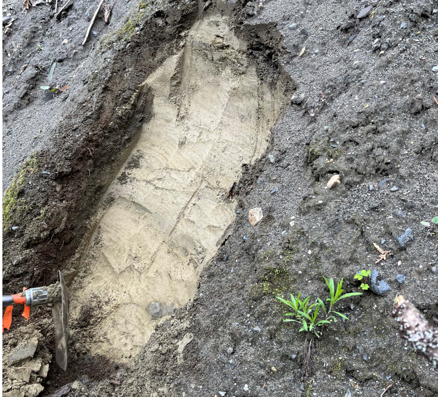
Figure 7: Photo taken on 5/8/2025 showing exposed glacial lake sands as well as overlying colluvium that was removed.
